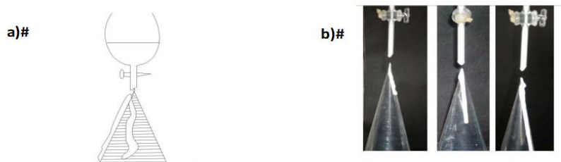
Fig.1. a) Cone system for measuring sliding index. b) Sliding of sample in consecutive stages.
