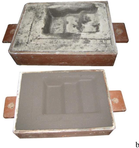
Fig. 2. Box mold: a - under face the mold with cement; b - under face the mold with gas oil.
